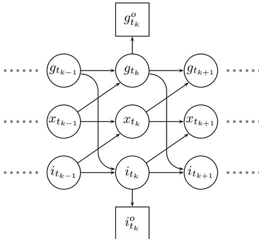
Figure 3. Directed acyclic graph illustrating the statistical dependencies for the latent processes,  $g$ ,  $x$  and  $i$ , and the observed processes  $i^o$  and  $g^o$ . The observed quantities are illustrated by rectangles and the unobserved quantities are illustrated by circles.
